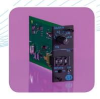
By way of example, with the amplifier normalised to 50pC/g a 10pC/g transducer rescales O/P1 to 2mV/g peak O/P1 level will increase from 1200 to 6000g (Vs =  $\pm 15V$ ).
